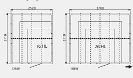
The dashed lines show the extent of the ceiling. The rooms can be extended further in the direction of the arrow. For other dimensions and versions, request a quote. Glass wall sections and service walls are available in the widths 398, 588 and 778 mm. They can replace corresponding sections in Excellent rooms at no extra charge.
